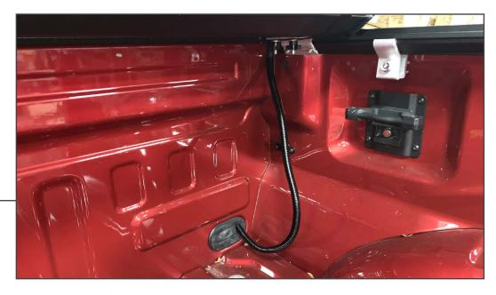
Fit (1) drain tube into the side rail fitting. Route the drain tube towards the vehicle bed grommet. Carefully cut a slot in the grommet to route the drain, or remove the grommet from the bed.
