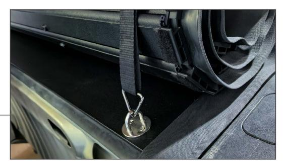
To store the tonneau cover, roll the tonneau cover towards the vehicle cab, and secure each side using the straps into the retainers in the tonneau cover panel. Ensure the straps are tightened after clipping into place.
