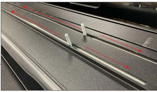
Fit the head of (4) M8 bolts into the front of the tonneau cover. Slide (2) bolts to the driver's side and (2) bolts to the passenger's side.
