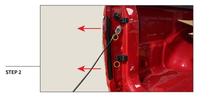
Remove (2) T-25 Torx screws from the side of the tail light. Pull the tail light firmly away from the vehicle to dislodge the (2) alignment pins inside the bed.
