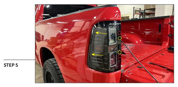
Align the (2) tail light alignment pins into the vehicle grommets. Then, secure the tail light to the vehicle bed using the original (2) T-25 Torx screws and (2) plastic push clips.
