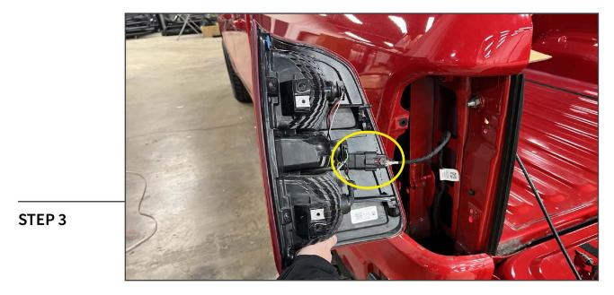
Slide the red connector lock back on the connector. Then, press the connector tab and unplug the vehicle electrical connector from the tail light harness.
