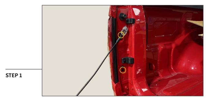
Lower the vehicle tailgate. Remove (2) plastic push clips from the side of the vehicle tail light.
