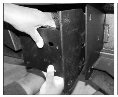
Step 1. Place supplied mounting bracket onto the bumper as shown. Line up the holes in the bracket with the holes in the bumper. Hold into position.
