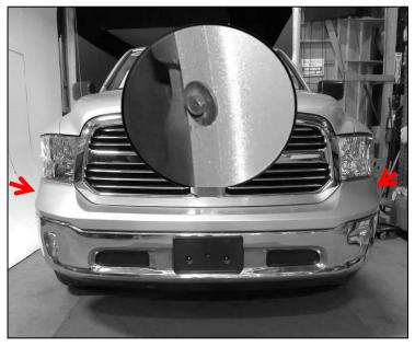
Step 3. Proceed to the inside of the vehicle wheel well. Using a 7mm socket locate and remove one factory hex head bolt holding the bumper cap onto vehicle. Set hardware aside for reinstallation.
