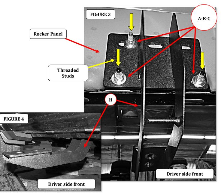
**Step-3** Locate the (3) threaded studs on the inner rocker panel at the center and rear of the cab and repeat step 2 to install two of the brackets using the supplied hardware. Note: The front mounting location is shown in Figure 3. The center and rear mounting locations are similar. Repeat steps for passenger side
