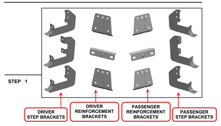
Please identify each mounting bracket using the engraved location identifier. Notice: The 4 sets Front and Rear step brackets & reinforcement brackets are the same. The 2 sets Center step brackets & reinforcement brackets are the same.
