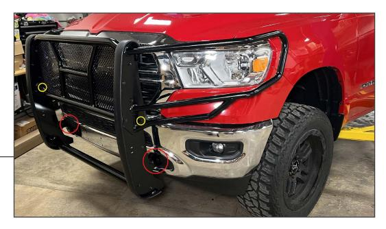
With assistance, fit the grille guard to the previously installed mounting brackets. Secure the bottom of the grille guard to the lower brackets using (4) M12 x 35mm bolts, (4) M12 lock washers, (8) M12 flat washers, and (4) M12 nuts. Then, secure the top of the grille guard to the upper brackets using (2) M8 x 35mm bolts, (2) M8 lock washers, (4) M8 flat washers, and (2) M8 nuts.
