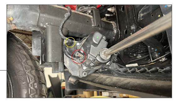
Safely lift and support the front of the vehicle off the ground. Locate the vehicle active shutter. Unplug the electrical connector from the motor. Then, use a panel removal tool to remove the harness retaining clip from the motor assembly.
