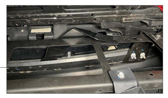
Fit the LH and RH upper mounting brackets (inner) through the gap between the bumper and grille. Begin at the center of the bumper, the brackets can be moved horizontally once in between the bumper and grille. Ensure the bracket appears similar to the diagram above.
