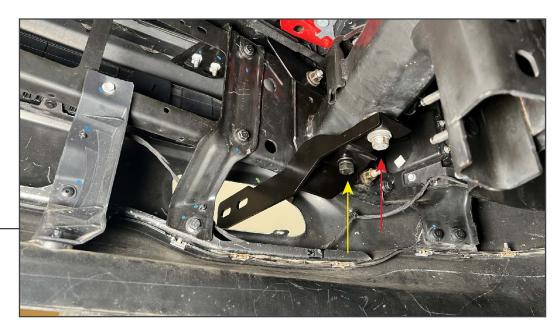
Fit the lower mounting bracket to the vehicle bolt. Secure the lower mounting bracket using (1) M14 x 35mm bolt, (1) M14 lock washer, and (1) M14 flat washer. Then, tighten the vehicle 18mm bolt.
