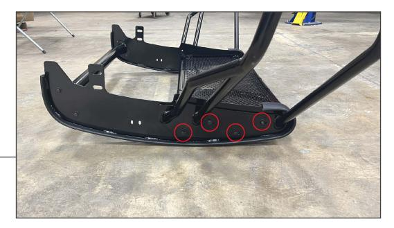
Fit the center grille guard panel in between the LH and RH bumper panels. Then, align each headlight guard to the center grille guard panel and the bumper panels. Once aligned, loosely secure the panels together using (8) M8 x 35mm bolts, (16) M8 flat washers, and (8) M8 lock nuts.
