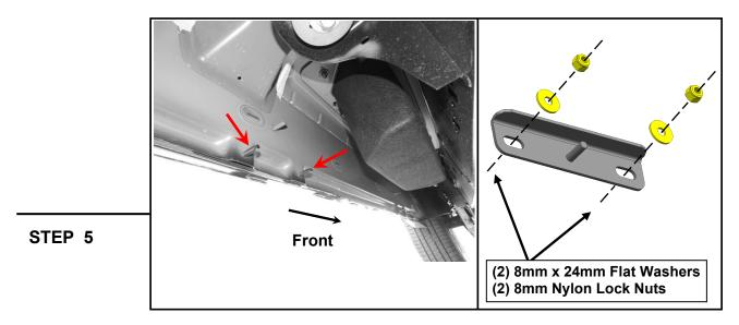
Loosely fit the (1) Driver Center reinforcement bracket to the (2) lower threaded studs using (2) M8  $\times$  24mm flat washers, and (2) M8 nylon lock nuts. Do not fully tighten to allow for later adjustments.
