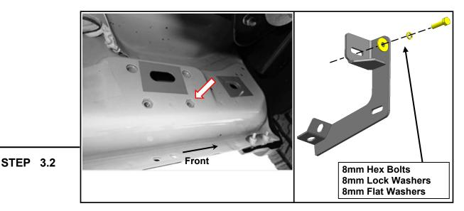
Start installation toward the front of the Driver/Left side of the vehicle.
