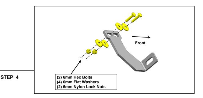
Loosely connect the (1) Driver Front reinforcement bracket to the back of the pinch weld using (2) M6 × 25mm hex bolts, (4) M6 × 22mm flat washers, and (2) M6 nylon lock nuts. Repeat this step for all Driver reinforcement brackets.
