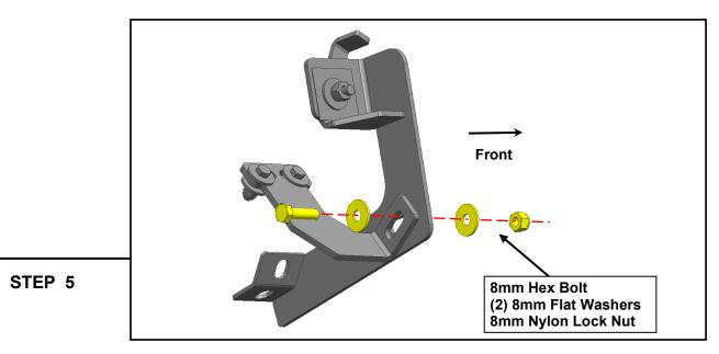
Loosely connect the (1) Driver Front step bracket to the (1) Driver Front reinforcement bracket using (1) M8 × 25mm hex bolt, (2) M8 × 24mm flat washers, and (1) M8 nylon lock nut.
