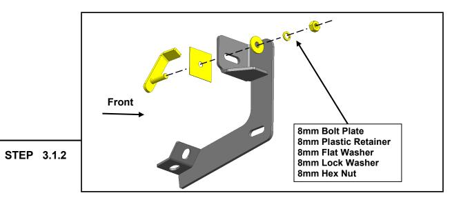
Thread (1) 8mm Plastic Retainer onto the threaded end and down tight against the body panel. **NOTE:** The Plastic Retainer is designed to keep the Bolt Plate from falling into the body panel and to aid in Bracket installation.
