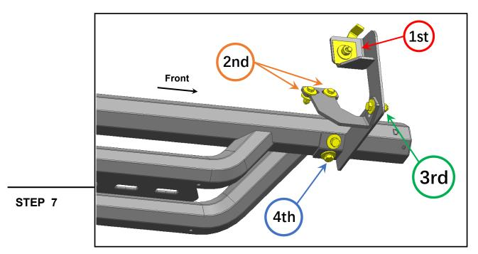
Tighten the mounting brackets to the vehicle. Adjust the Drop Step to the desired angle, and tighten the M8 combo bolts to secure the step into place. See photo for tightening order visual.
