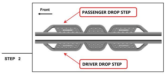
Identify each drop step by identifier on the front. Notice: "D" for Driver/Left Side; "P" for Passenger/Right Side.
