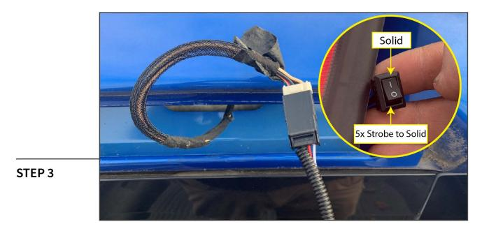
Plug in the brake light electrical connector into the vehicle's wiring harness. Toggle the switch to enable 5x strobe feature.
