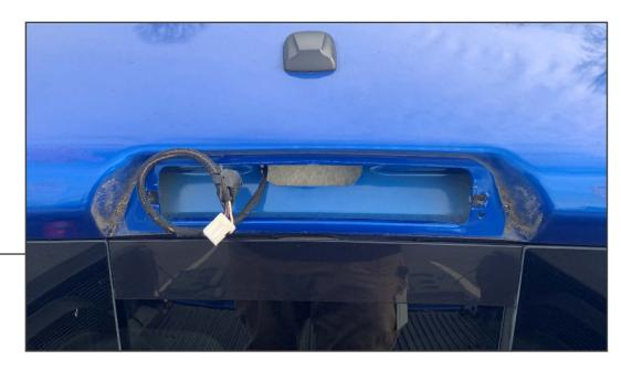
With the screws removed, remove the brake light from the vehicle using a plastic pry tool. Unplug the electrical connector from behind the brake light.
