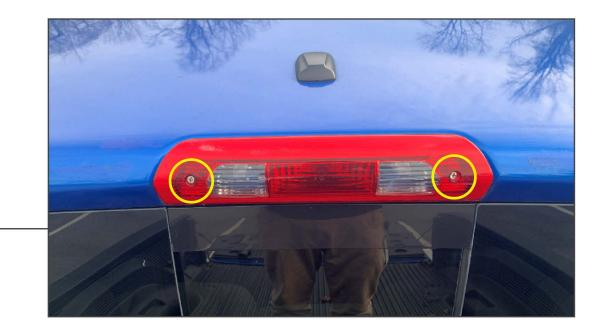
Remove (2) Phillips head screws from the third brake light assembly.
