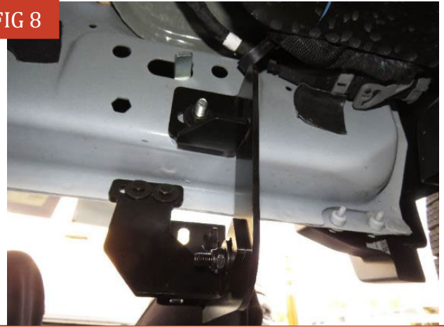
(Fig 8) Driver/Left Mounting Bracket and Support Bracket attached to the Front Mounting Location.
