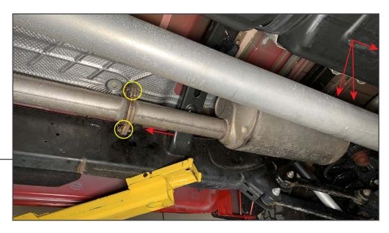
Remove (2) 16mm bolts from the front muffler flange to disconnect the muffler from the front portion of the vehicle exhaust. Disconnect the (3) muffler rubber hangers, and (1) LH tailpipe rubber hanger, then remove the exhaust assembly from the vehicle.
