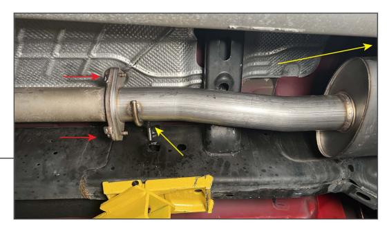
Align the muffler assembly to the vehicle exhaust system flange, and insert the (3) metal hangers into the vehicle rubber/polyurethane hangers. Thread the original (2) 16mm bolts into the flanges, but do not fully tighten to allow for later adjustment.
