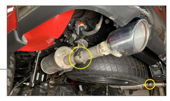
Lift and support the vehicle using a floor jack and jack stands. Locate and remove the (2) exhaust tip pipes from the exhaust by loosening the exhaust clamps.
