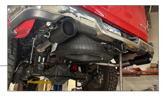
Fit the (2) exhaust tips to the exhaust system. Adjust the exhaust system to best fit the bumper cutouts, and tighten each exhaust clamp to 45 ft. lbs.
