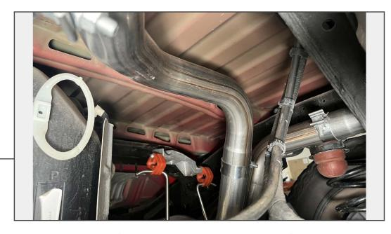
Insert the LH over axle pipe into the muffler assembly, and secure but do not fully tighten the exhaust clamp to secure the pipe into place.
