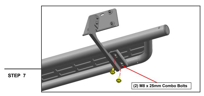
With all brackets loosely mounted to the vehicle, fit the running board onto the brackets, and loosely secure into place using (6) M8 x 25mm combo bolts.
