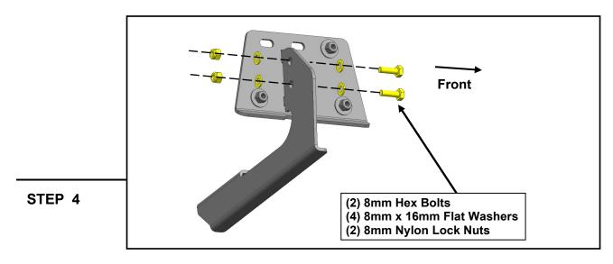
Loosely connect the (1) Driver Front step bracket to the (1) Driver Front reinforcement bracket using (2) M8 × 25mm hex bolts, (4) M8 x 16mm flat washers, and (2) M8 nylon lock nuts.
