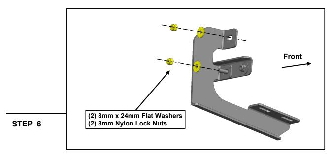
Loosely connect the (1) Driver Center step bracket to the (1) Driver Center reinforcement bracket using (2) M8 × 24mm flat washers, and (2) M8 nylon lock nut.
