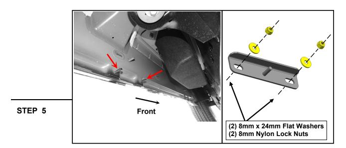
Loosely fit the (1) Driver Center reinforcement bracket to the (2) lower threaded studs using (2) M8  $\times$  24mm flat washers, and (2) M8 nylon lock nuts. Do not fully tighten to allow for later adjustments.
