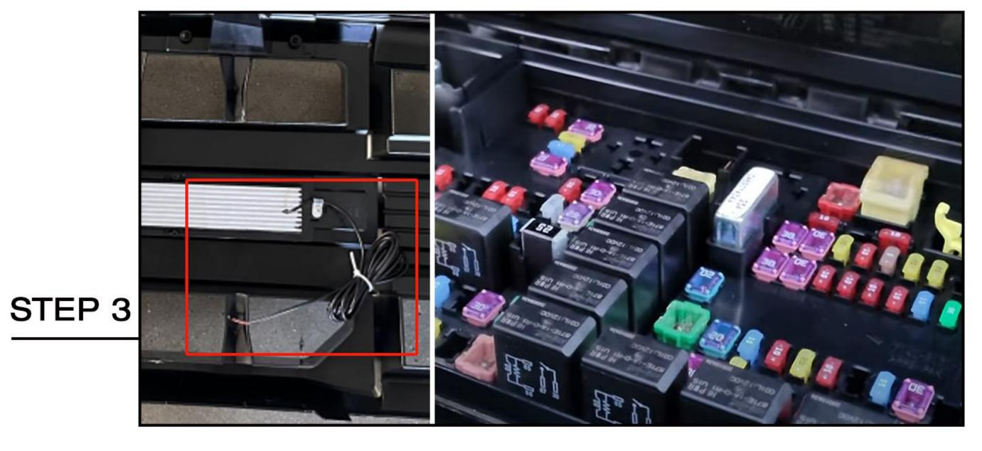
DRL Wiring: Wire to fuse box, the red wire connects to the ACC, the black wire connects to the negative of battery.
