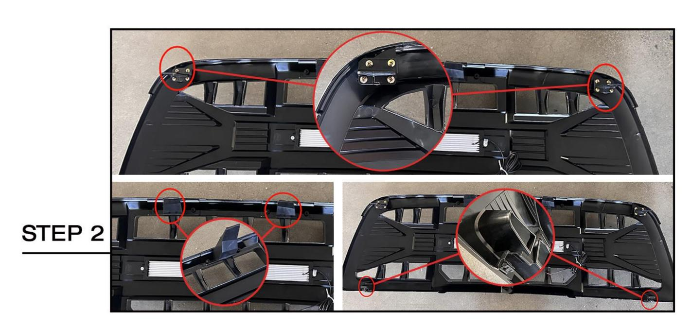
Install 4 mounting brackets.(2 on each end and 2 in the middle).Install 2 metal clips on each end.
