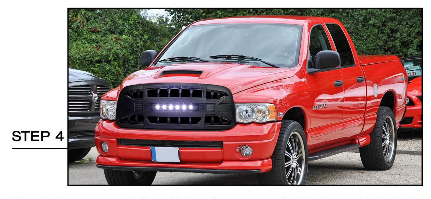
Align the bottom metal clips with the slot, top mounting brackets with the hole on the car. Get these snapped in, screw all bolts and clips to complete the installation.
