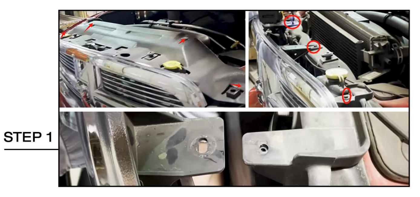
Open the hood,remove 4 clips(2 in the middle and one on each end)with a pry tool to remove shroud cover from vehicle. Remove 3 bolts with an impact wrench and swing the grille to remove the original grille.
