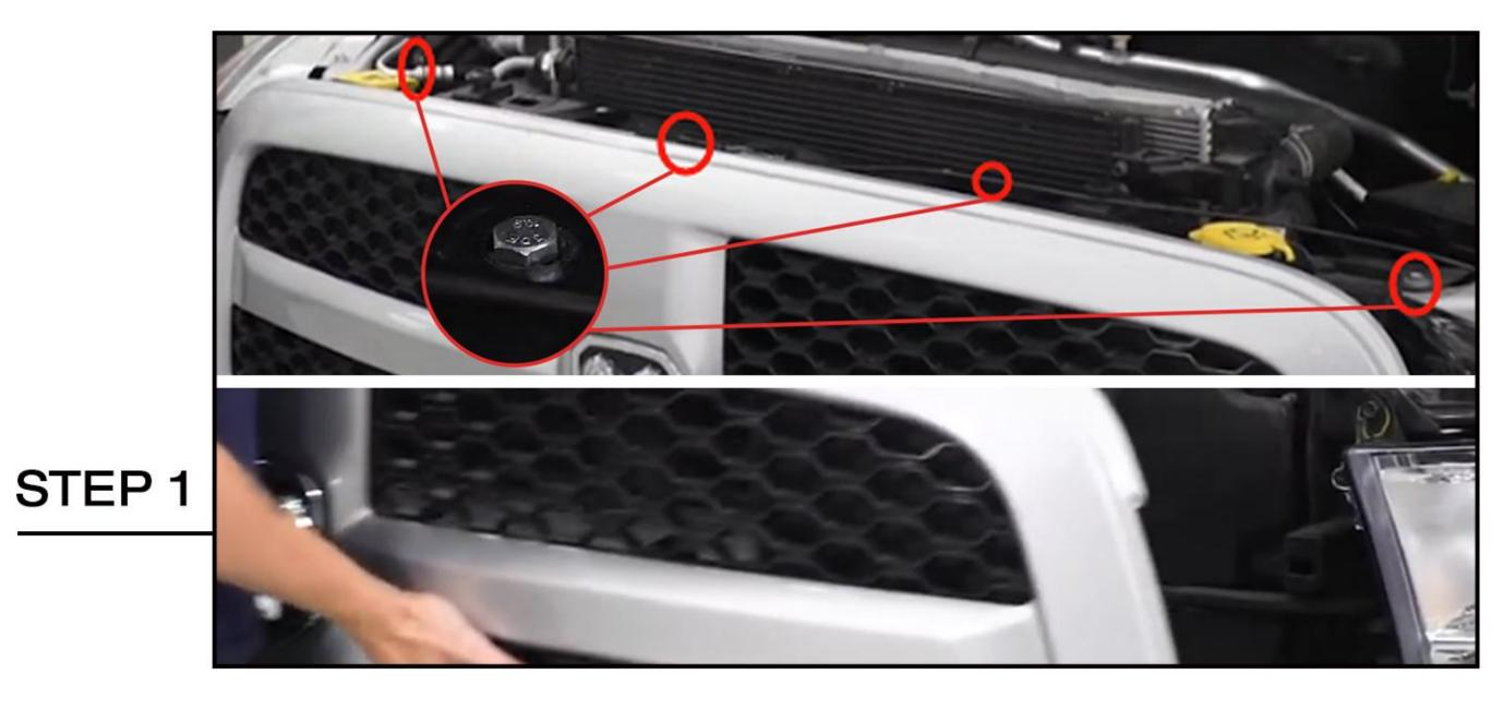
Remove the 4 10-millimeter bolts holding on the top of the grille with a 10-millimeter socket. Then lift up on the brackets and pull straight out towards you to remove the grille.
