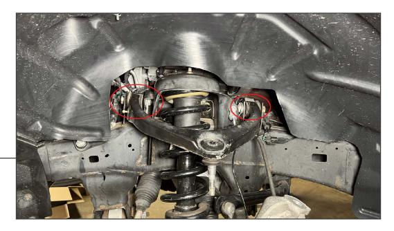
Remove (2) 21mm bolts and flag nuts from the upper control arm to the vehicle frame. Remove the control arm from the vehicle.
