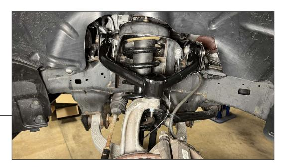
With the vehicle suspension loaded, torque the upper control arm bolts evenly to 128 ft. lbs. Installation is now complete.
