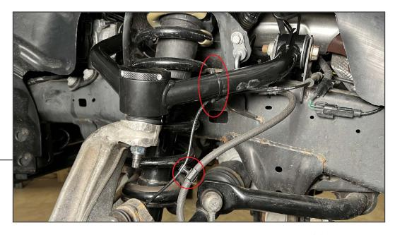
Secure the upper control arm ball joint to the steering knuckle using the included (1) 19mm lock nut. Secure the ABS line to the control arm using (1) cable tie and the original brake hose retainer.
