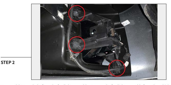
Remove (3) 10mm bolts from the fog light assembly. Remove the fog light assembly from the vehicle.
