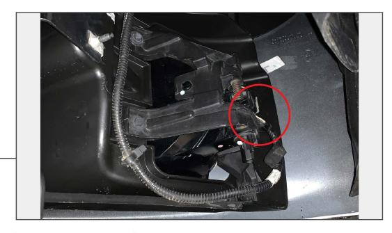
From behind the front bumper, unplug the fog light electrical connector.
