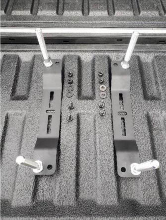
1. Select correct mounting pins for chosen recovery boards.
