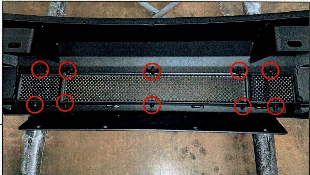
Secure the LH, RH, and Center mesh panels to the bumper using (10) M6 x 20mm combo Allen bolts and (10) M6 flange nuts.
