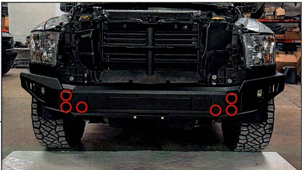
With a helper, lift the new bumper to the vehicle, and secure into place using (6) M12 x 35mm bolts, (6) M12 lock washers, (12) M12 flat washers, and (6) M12 nuts.
