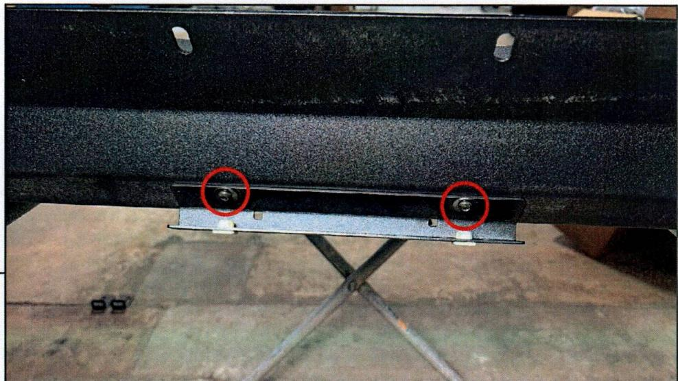
If desired, secure the front license plate mounting bracket to the bottom of the bumper using (2) M6 x 20mm Allen bolts, (4) M6 flat washers, and (2) M6 lock nuts. Then, fit the (2) square plastic screw retainers into the square holes in the bracket.
