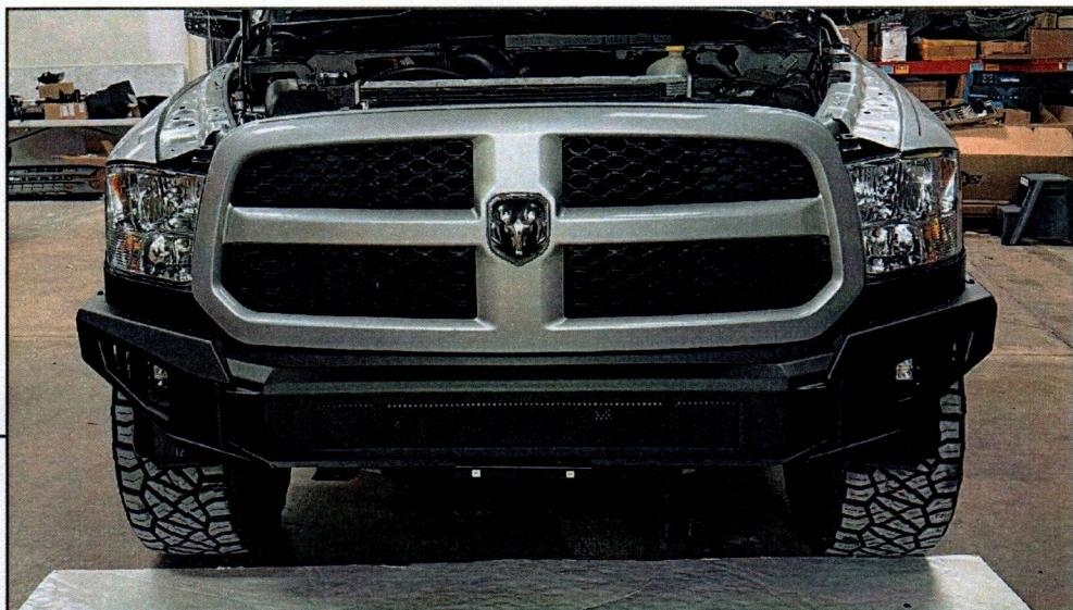
Fit the grille and radiator cover panel to the vehicle reusing the original hardware.
