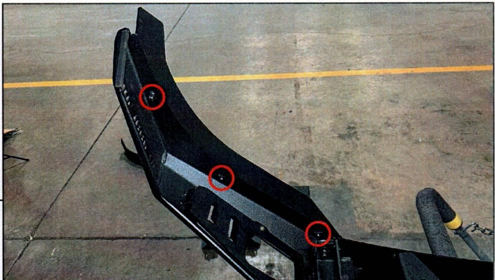
Fit the LH and RH upper panels to the bumper, and secure using (3) M6 combo Allen bolts, (3) M6 flat washers, and (3) M6 flange nuts. Do not fully tighten the bolts to allow for adjustment after the bumper is installed to the vehicle.
