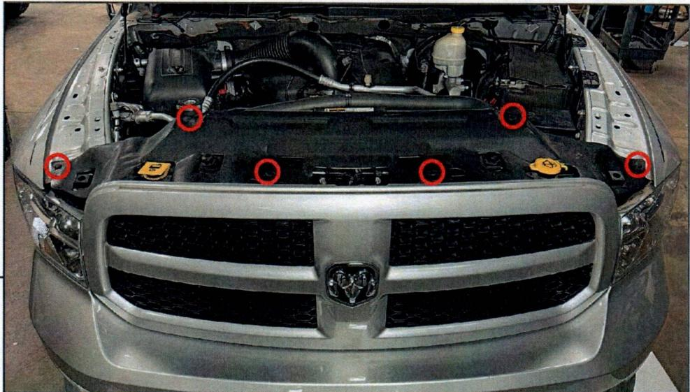
Open the vehicle hood. Remove (6) plastic push clips from the radiator cover, and remove the cover from the vehicle and set aside.
