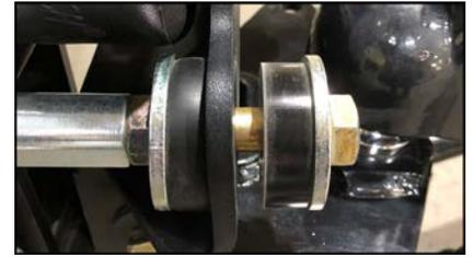
Figure 13: Hitch frame resting on bump cushions closer to tailgate - add air.
