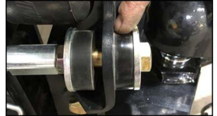
Figure 14: Hitch frame resting on bump cushions closer to trailer - stop adding air.
