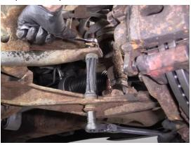
If you can't prevent the link or joint from spinning, you may need to cut the link free. Your cutting wheel can access it closely to do it, but take care not to contact any other parts like brake lines, calipers or CV joints.
