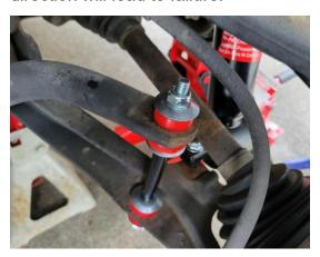
Position the new link and start the nuts on the ends of the link, then tighten the nuts. Use a torque wrench to finish the job, tightening them to at least 20 Ft  $\cdot$  lbs  $(27 \text{ N} \cdot \text{M})$ .
