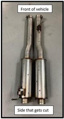
2. Mark 1-13/16" of an inch after the resonator with tape or a marker as shown for a cut line.
