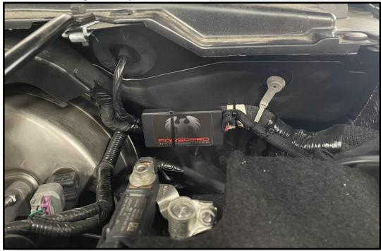
10. Continue running the wiring down the driver's side of the engine bay, to the top of the frame rail.
