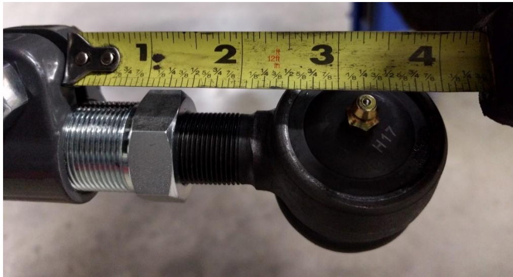
Figure 10. Tie Rod End Adjusted MAX 3.25" Out (Double Adjuster Side)
