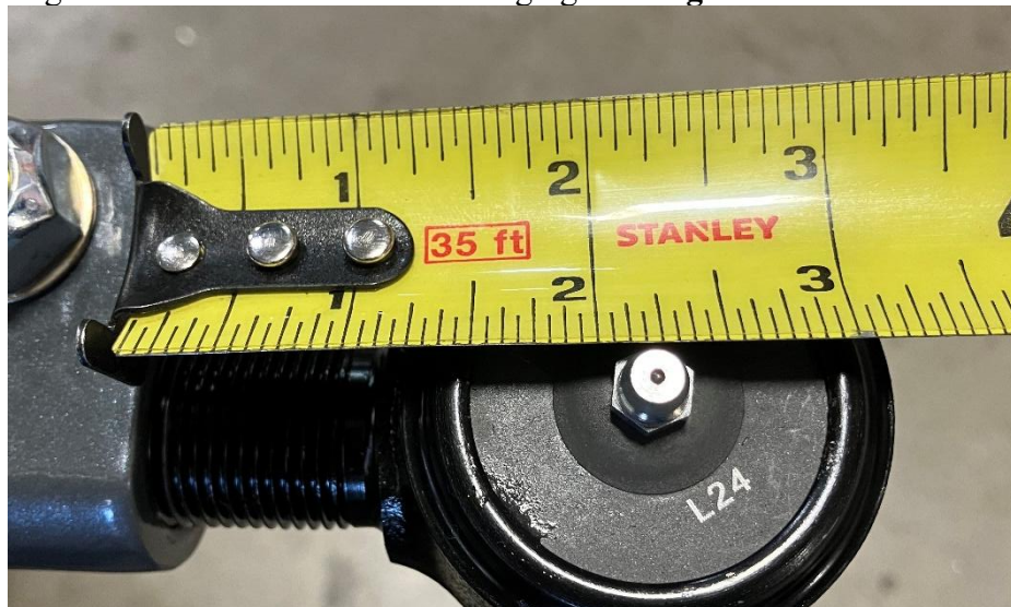
Figure 4. Passenger Side TRE Adjusted to 2 1/4" From End of Tie Rod Forging.
