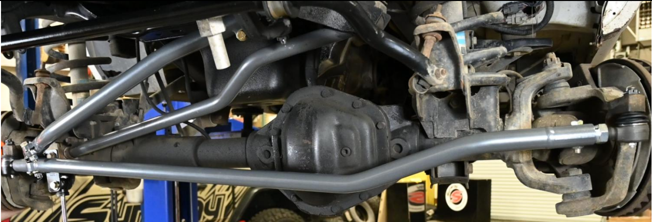
Figure 16. Installed Tie Rod and Drag Link
