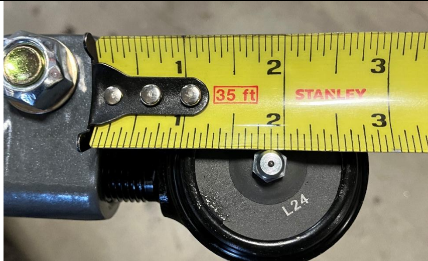
Figure 5. Passenger Side TRE Adjusted to 1 7/8" From the End of Tie Rod Forging.
