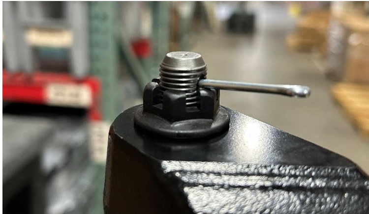
Figure 7. Cotter Pin Not Engaged in Castle Nut Slots
