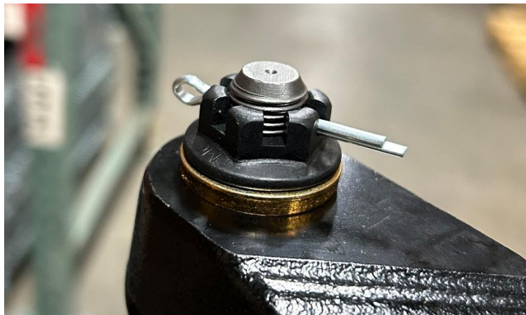
Figure 8. Washer Installed to Engage Cotter Pin and Castle Nut Slots
