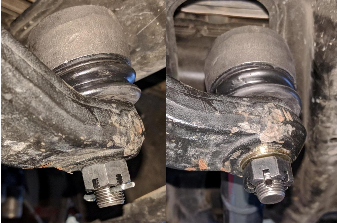
Figure 18 and 19. Washer Used Under Castle Nut
