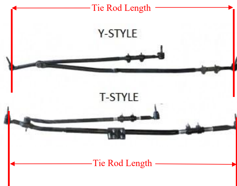
Figure 1. How to Measure Tie Rod Length
