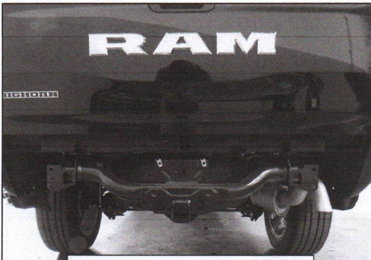
(Fig 5) Bumper completely removed
