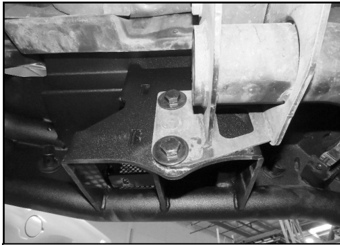
(Fig 19) Passenger side of the Rear Bumper attached to the factory hitch
