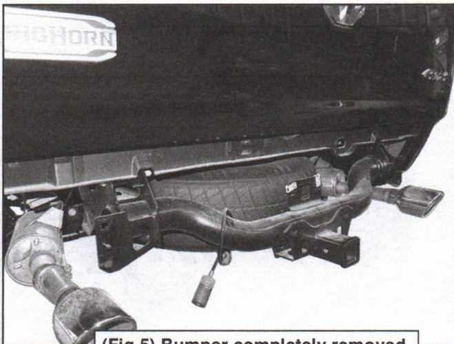
(Fig 5) Bumper completely removed
