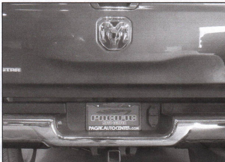
(Fig 1) Remove the license plate in order to access the two bolts holding the bumper
