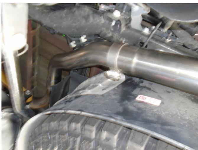
**Step 6:** Loosly install the two Tailpipe Extension Pipes using the supplied clamps. The longer, three bend pipe will be for the drivers side.
