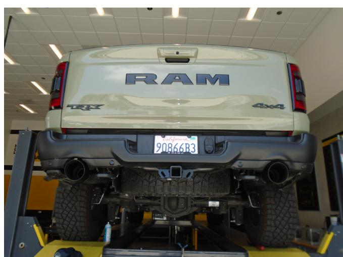
**Step 8:** Once a final position has been chosen for the new exhaust system, evenly tighten all clamps and fasteners, from front to rear, using the torque specifications on page one of the instructions. Inspect all fasteners after 25-50 miles of operation and re-tighten if necessary.
