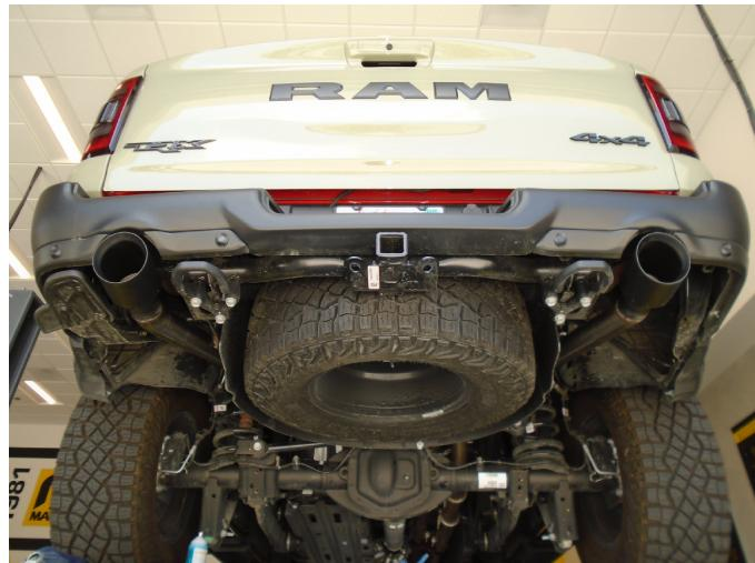
**Step 7:** Loosely attach each Tail Pipe Assembly to the Tailpipe Extension Pipes using the supplied clamps. Locate the welded hangers to the rubber isolators.
