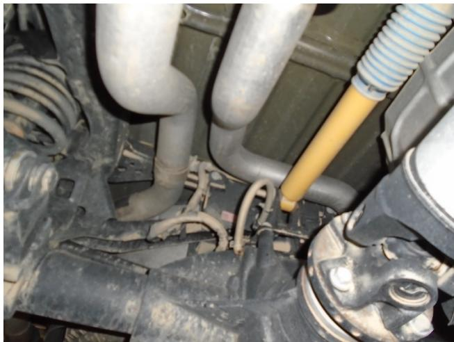
**Step 2:** To remove the system you will need to either cut the OE system with a Sawzall or similar cutting tool, or remove the rear shock absorber attached to the rear differential. The system may now be removed.
