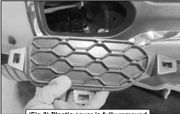
(Fig 3) Plastic cover is fully removed
