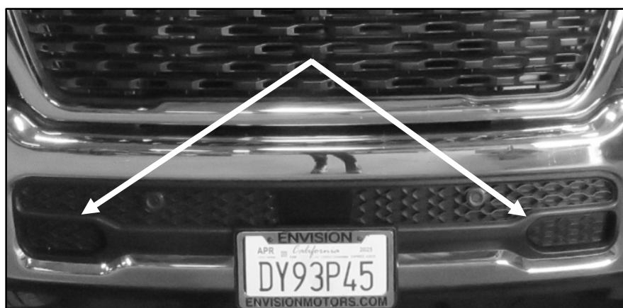
(Fig 1) Vehicles that do not come equipped with tow hooks will need to remove the plastic covers
