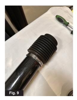
Install the Short Coupler (C) onto the turbo with the two Hose Clamps (H). (Fig. 10)
