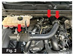
Remove the bolt securing the intake tube to the engine.
