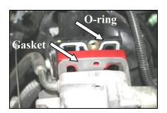
6. Place one fiber gasket (#4) between the Poweraid spacer (#1) and the throttle body. Make sure the flat face of the Poweraid spacer is against the throttle body with the bore extending into the intake manifold. Use caution to retain the factory o-ring gasket on the intake manifold.
