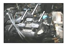
**5.** Install three 1/2" extension plates (#5) using the provided flat head countersunk bolts(#6). Point the long end towards the radiator, and snug them down.
