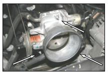
**2.** Using a 10mm socket, remove the three nuts that hold the throttle body to the intake manifold.
