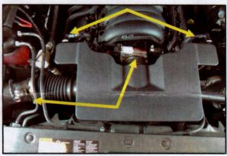
**5**. Reinstall the intake system and tighten the two hose clamps. Reconnect the valve cover breather lines.
