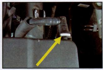
2. The guick connects for the valve cover breathers are removed by depressing the grey locking tab in the fitting and sliding
