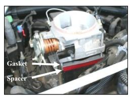
5. Place the fiber gasket (#9) between the Poweraid spacer (#1) and the throttle body. Make sure the flat face of the Poweraid spacer is against the throttle body with the bore extending into the intake manifold. Use caution to retain the factory o-ring gasket on the intake manifold.
