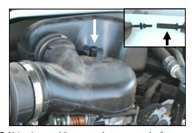
7. Using 6mm and 8mm wrenches, separate the factory rear throttle body stud as shown (reuse the top). Install the top of the stud onto the rear throttle body stud. Re-install the intake hat hold down nut. Tighten all bolts securely.
