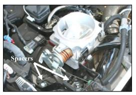
6. Install one 1/2" round spacer (#5) under each hole in the throttle cable bracket. Install the 6mmx 30mm bolt (#4) in the front hole, and the 6mmx 35mm bolt (#5) in the rear hole. Re-install the throttle cable bracket and nut onto the front of the throttle body. Install one 6 mm washer (#6) and 6mm nut (#7) onto each of the three throttle body studs. Tighten all bolts and nuts securely. Reconnect the harness plugs on the throttle body.
