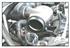
2. Disconnect the breather hose elbow from the intake hat. Remove the intake hat, and hold down nut, and save them for reuse.
