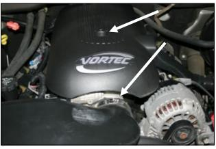
1. **Disconnect the negative battery cable.** Loosen the bolt that secures the beauty cover to the engine and remove it and the cover from the vehicle. Loosen the hose clamp that secures the factory air intake tube to the throttlebody.
