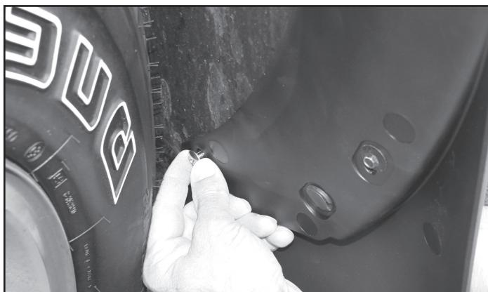
**7** Insert (1) of the supplied bolts through the innermost hole of the MudFlap, the plastic liner and metal behind it. Using (1) of the supplied nuts, reach behind the MudFlap, and attach the nut to the bolt with the serration on the nut towards the head of the bolt. Hand-tighten the bolt and nut.
