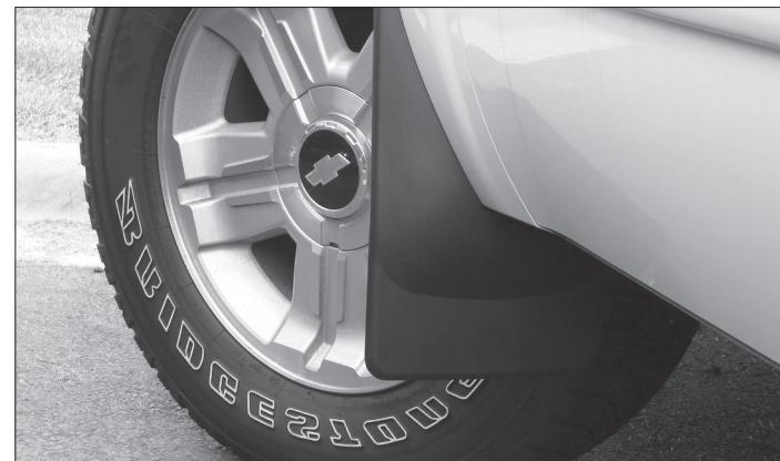
**9** Begin passenger side installation by parking the vehicle on the level surface with the wheels turned fully to the right. Repeat steps 3-8.
