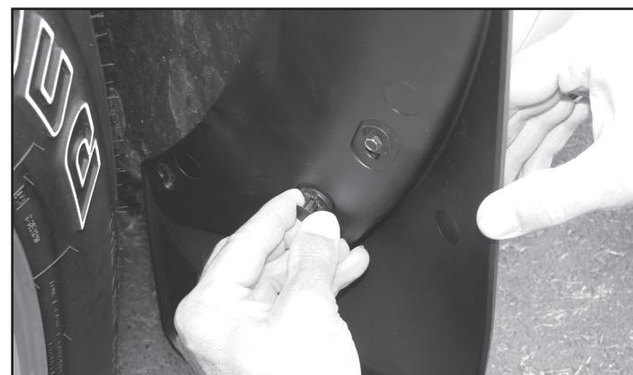
**6** Place the outer body of (1) of the previously removed plastic rivets completely through the MudFlap and the hole in the fender. Firmly press the rivet body completely through the MudFlap and into the hole to ensure that the rivet body is snug against the MudFlap. While holding the rivet body tightly to the MudFlap and against the fender, place the inner core of the rivet into the body and firmly press in the inner core.
