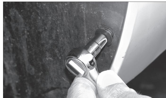
**8** While pressing the MudFlap snug against the fender, tighten the (2) hex head screws, the previously installed Phillips head machine screw and nut.
