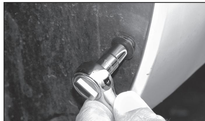
**4** Remove the (2) hex head screws holding the plastic fender liner. Save these screws for reuse.
