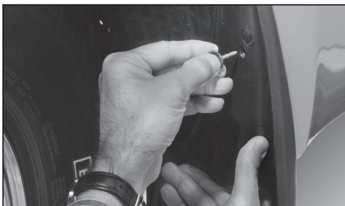
**5** Press the MudFlap against the fender for a tight fit. Insert and snug the hex head screws removed in step 4. **IMPORTANT** - Do not fully tighten at this time.
