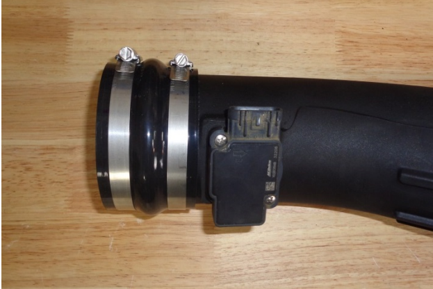
19. Install two screw clamps (8) on the flex coupler (11), and install the coupler on the filter end of the intake tube. Snug (but do not yet tighten) just the clamp on the tube, and leave the other clamp loose.
