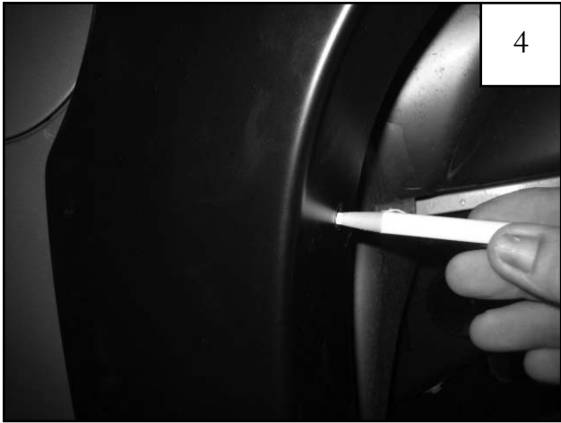
Holding flare in position on fender, use a grease pencil to mark six hole locations.
