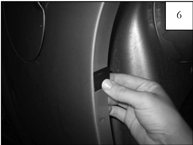
Center a supplied black plastic tab over each mark made in Step 3, aligning edge of tab with inside of fender lip (tab may extend over outside of fender).
