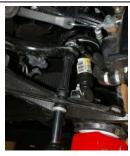
20. Re-attach the brake line bracket to the control arm and insert the wheel speed sensor cable into each of the factory harness clips. Repeat steps 3-20 on driver side. Make sure all hardware is tight and torqued to factory specs. Install the front wheels and torque the lugs to factory specs. Lower the vehicle and install the skid plate.
