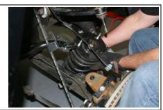
12. Install the new strut extension spacer onto the top of the factory strut. Unlike some kits, you don't need to cut the studs off or swap the struts from side to side. The ReadyLift aluminum spacer is designed to provide the necessary lift while retaining the use of the factory strut studs. This is a great advantage should you ever want to return the vehicle to stock such as with a lease vehicle.
