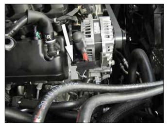
3. On vehicles equipped with the intake plenum support bracket, install the provided spacer between the bracket and cylinder head and secure with the provided hardware.
