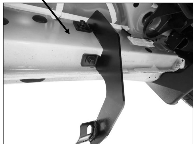
(Fig 4) Driver/left front Bracket installed
