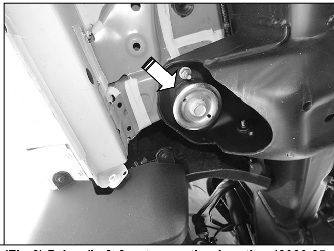
(Fig 2) Driver/Left front mounting location (2020 25-3500 model with cupped body bolt washer shown)
