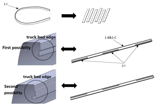
5. Place the side rail on the bed rail, and push it to the front wall of truck bed. Place one clamp at the front of the side rail and one at the rear (please make sure the rear clamps is placed on the position that is closest to tailgate). Tighten the clamps each side.
