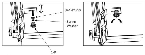
$\times$ ATTENTION: Make sure the Flat Washer and Spring Washer are all placed on bolt before screw the plastic nut on.
