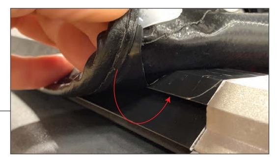
Fold the tonneau cover out towards the rear of the vehicle. The black plastic portion of the tonneau cover clips into the outer edge of the rail. Hook the cover into the rails. Work from the front to the back on both sides.
