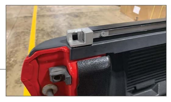
Place the rails on either side of the bed. Note the orientation of the locking portion of the rail shown.
