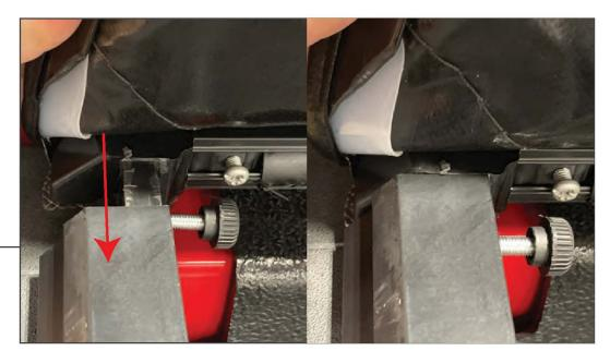
Slide the tonneau cover into the rails at the front of the bed. The plastic portion slides into the bed rails on both sides of the vehicle. Use the thumb screw to secure the tonneau cover to the rails.
