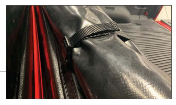
When the tonneau cover is not in use, fold back the tonneau cover. Remove the center support bars and use the nylon straps to lock the cover in position.
