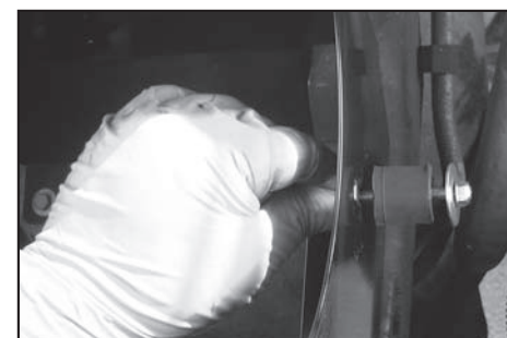
Step 9 Place the rubber vibration mount, fender washers and M6 lock nuts on the side of the housing as shown. Do not tighten the bolts at this time.
