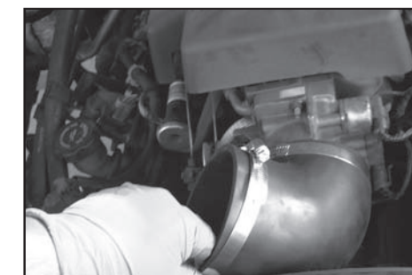
Step 10 Slide the 4" angled coupler and two 4" hose clamps over the throttle body. Do not tighten the clamps at this time.
