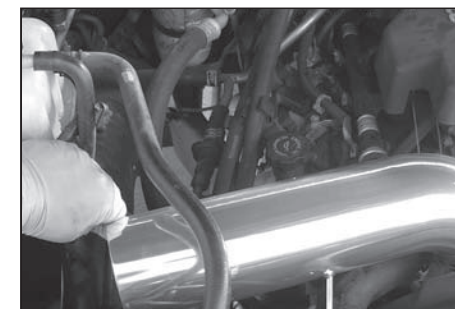
Step 11 Place the intake tube in the engine compartment. Slide the lower angled bracket between the vibration mount and the housing.
