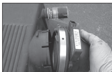
Step 6 Loosen the hose clamp securing MAF sensor to the air box. Carefully remove MAF sensor and rubber ring from the air box assembly and set aside for later use.
