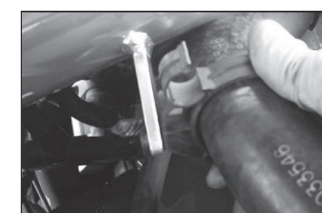
Step 12 Insert the radiator hose bracket into the bracket on the side of the intake tube.
