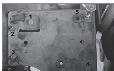
Step 7 Remove the five 10mm bolts securing the lower air box tray and remove tray. Set the bolts aside as they will be reused later.
