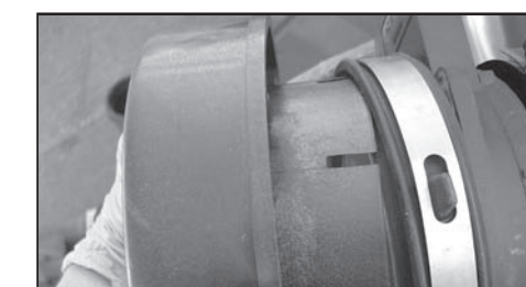
Step 14 Attach the MAF sensor and OE rubber ring to the MAF adapter. Slide the adapter between the rubber ring and the tabs as shown. Secure MAF sensor to the adapter with the OE hose clamp.
