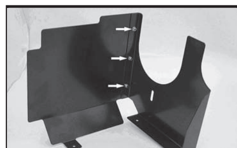
Step 8 Using the included 5mm Allen bolts, lock nuts and washers, assemble the heat shield as shown. Install the Allen bolts from the outside of the shield and put the flat washer and lock nuts on the inside. Once all the hardware is installed, use the included hex key wrench and an 8mm (5/16" will also work) wrench to fully tighten all of the lock nuts. Place the filter shield in the engine compartment. Secure the shield with the air box tray bolts removed in step 7.
