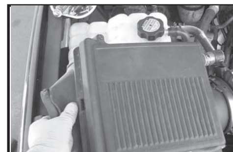
Step 5 Grab the air box from both sides and pull up and out. The air box is held in place with rubber grommets
