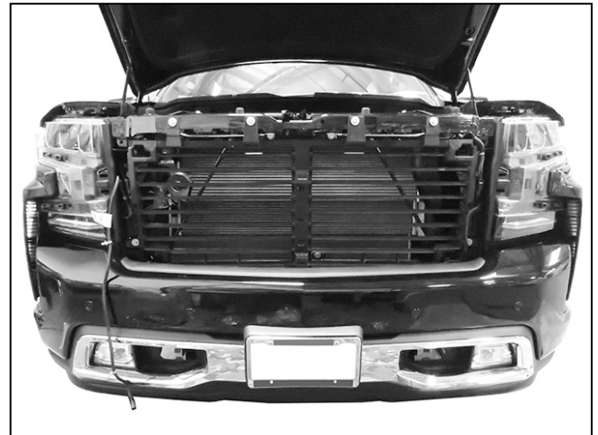
(Fig 2) Firmly pull grille straight out from vehicle
