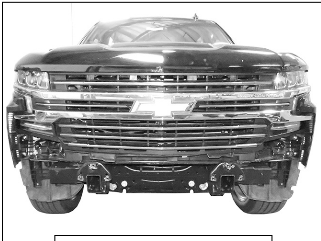
(Fig 7) Reinstall grille and cover
