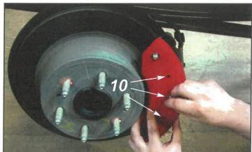
10. Align the rear caliper covers over the mounting brackets and install the supplied flat washers, lock washers and 1/4-20 x3/4" allen head bolts into the pre-installed 1/4-20 cage nuts on the mounting brackets.
