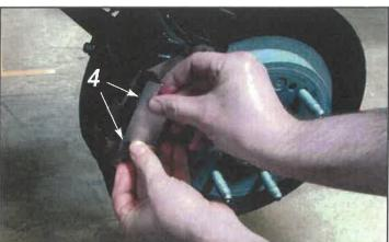
4. Align the front caliper cover spacer bracket tabs into the slots in the base mounting brackets installed in the previous step. Push in on the front caliper cover spacer brackets until the mounting tabs make contact with the face of the factory calipers.
