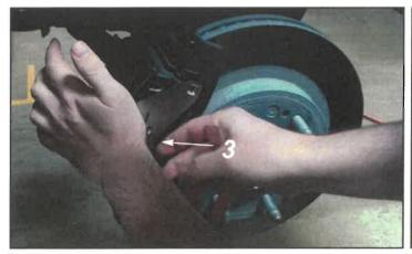
3. Push the face of the front caliper cover base mounting brackets down until the pre-installed cage nuts fit over the face of the calipers. IMPORTANT: On some models, you may need to pull the bracket from the bottom to keep the cage nuts from catching on the face of the caliper.
