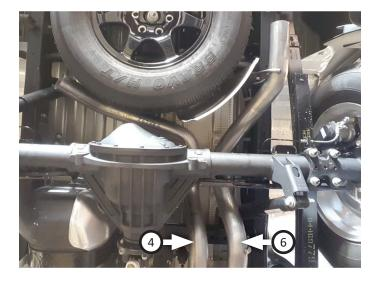
13. Place clamp (7) onto left rear tailpipe (5) then connect it to left front tailpipe. Insert wire hanger into rubber hanger then tighten clamp just enough to hold parts.
