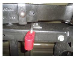
12. Route **left front (4)** and **right tailpipes (6)** over axle and connect them to muffler. Insert wire hangers into isolators then tighten clamps just enough to hold parts.
