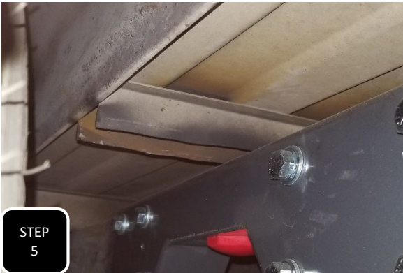
Step 5 Before being able to test fit the frame support, you may need to trim the bed rib, directly above, if your truck is equipped with one. Using a suitable cutting device, trim the bed rib about 1/2" up from the bottom. Trim from the end of the rib to at least the inside edge of the frame to ensure an easy install of the frame support and no contact of the two.
