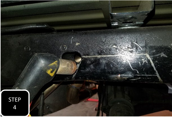
Step 4 Cut out the scribed line using a plasma cutter or other suitable cutting device
